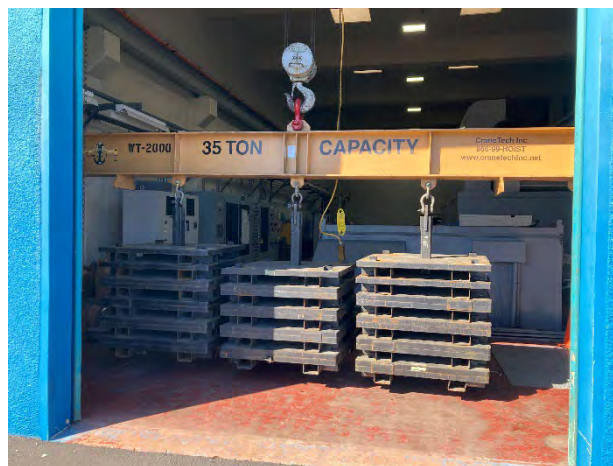
OLEPS Overhead Crane Quadrennial Load Testing
