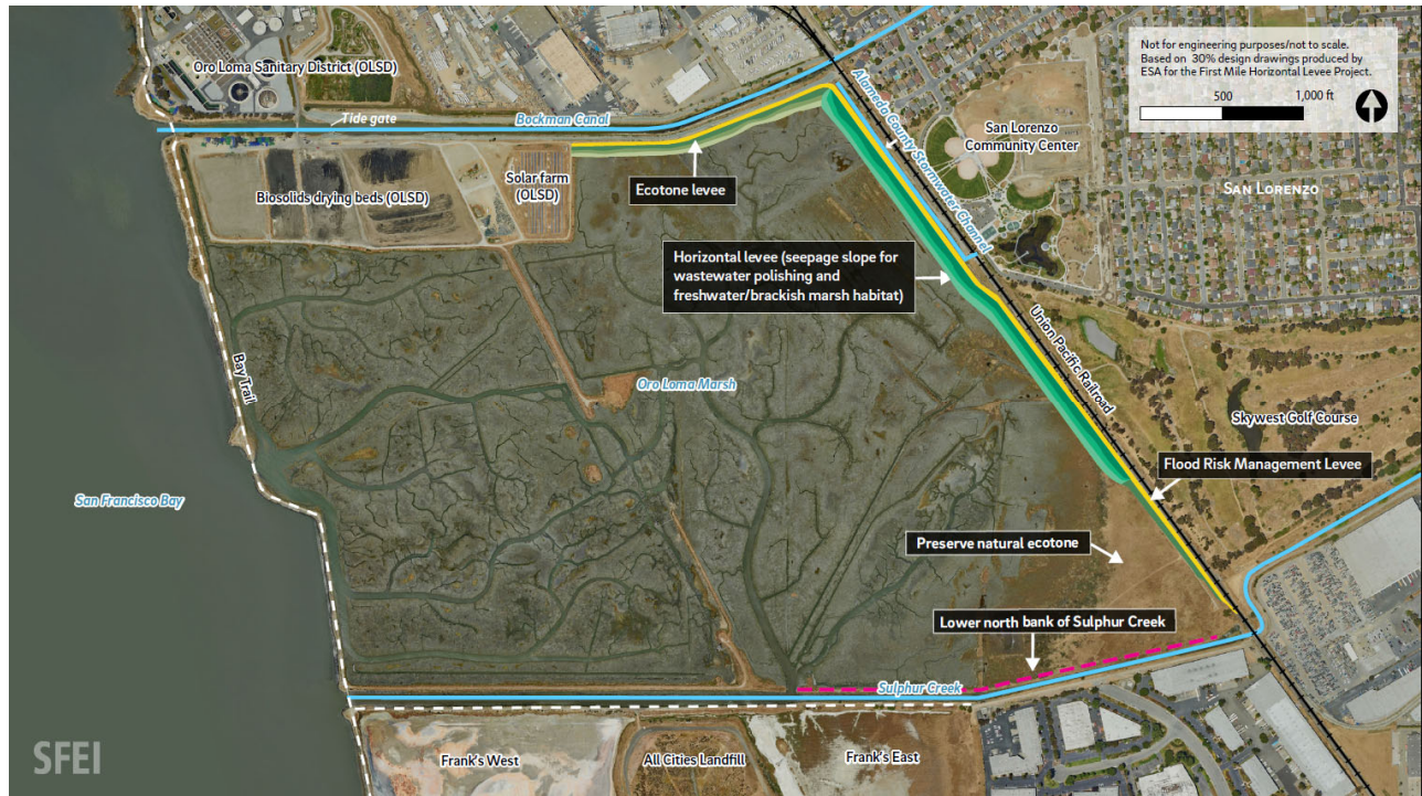
Figure 2 – First Mile Horizontal Levee Illustration
