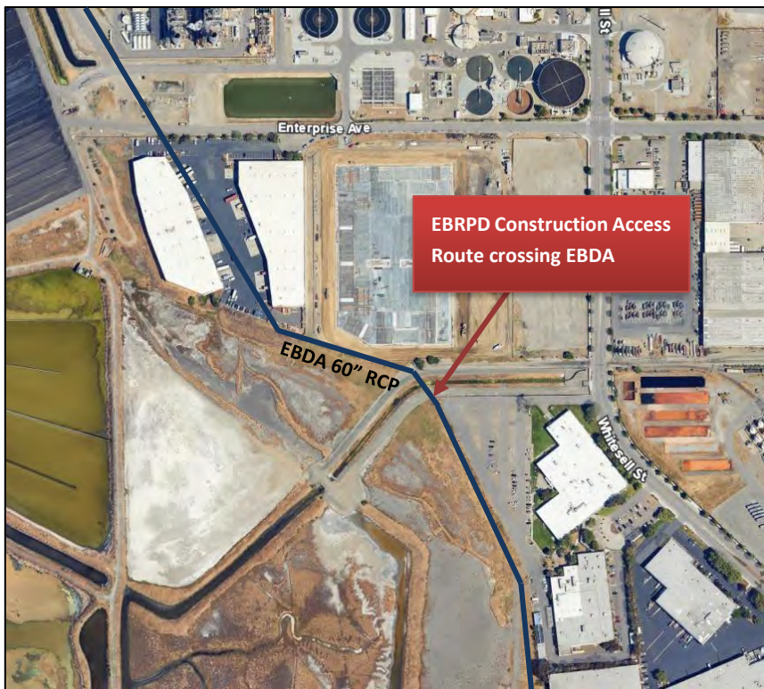
Figure A – Location of EBRPD Construction Access Route to Whitesell St. crossing over EBDA’s 60-inch RCP force main pipeline. The Construction Access Route will be on the south side of the drainage channel west of Whitesell St.
